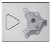
9. Remove the suction flange (39) and flange o-ring (38). Inspect the o-ring for wear and replace as necessary.
